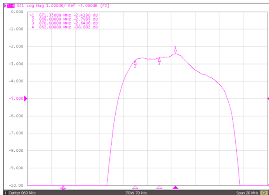
S21 response: (Span 20 MHz)
