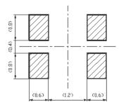
**Note:** This package has two extra pads in the middle (pin #5 and #6) that are used to test the internal Xtal by the factory, but are not intended for customer use. Do not place ground (GND) patterns (including ground pads, via holes, etc.) under the crystal unit, especially under pin #5 and #6. Also, do not run RF signal power or digital line under the package in the multi-layered PCB.
